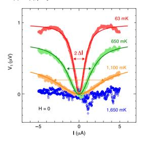
**Fig. 3.** The anomalous nonlinear voltage (ANV) which is described by the voltage  $V_1$  is extracted from *I*–*V* characteristics in Fig. 2, where the lines are Lorentzian fitting curves. The half-widths  $\Delta I$  of the fitting curves are represented by two-headed arrows. We eliminated the offset voltage of 0.13  $\mu$ V in order to discuss the ANV.
