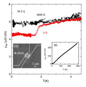
**Fig. 1.** Temperature dependence of resistivity of submicron  $Sr_2RuO_4$  in zero magnetic field (0 G) and in a magnetic field (H = 3000 G) applied parallel to the *c* axis. Flat tail resistivity can be seen at low temperatures below  $T_c = 1.69$  K. Inset (a) shows a micrograph of a submicron  $Sr_2RuO_4$  single crystal connected to gold electrodes. Inset (b) displays the temperature dependence of the resistivity in the *ab* plane from room temperature down to 4.2 K.
